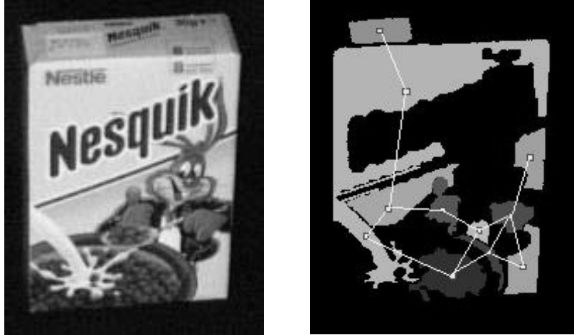
Fig. 1. a) an image of the object b) the image components represented in a graph
